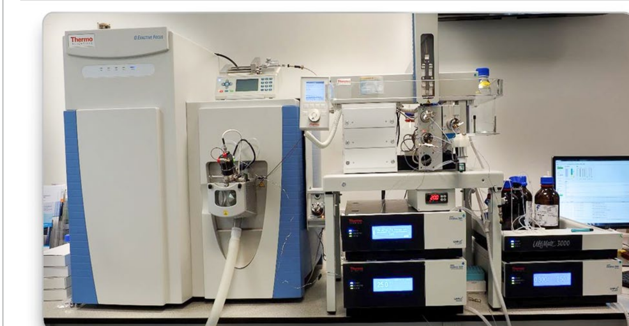
Figure 2. Q Exactive Focus Mass Spectrometer, showing EQuan On-Line SPE System.
