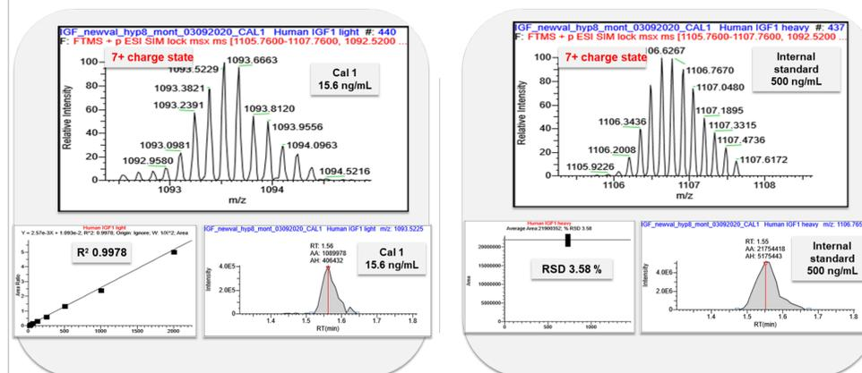
**Figure 3. EASY-IC enable IGF-1 mass accuracy within  $\pm 0.8$  ppm in Calibrators and  $\pm 1$  ppm in serum samples across 130 hours of non-stop run time.**
