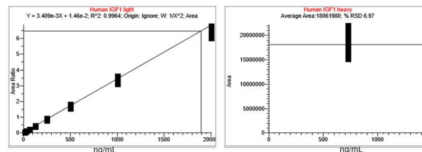
**Table 1. Robustness statistics for replicates (n=54) of a calibration curve across 130 hours of non-stop run time for IGF-1.**
