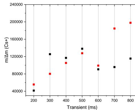
Fig. 3b: Mass resolution vs. transient length after zerofilling and hanning apodization
