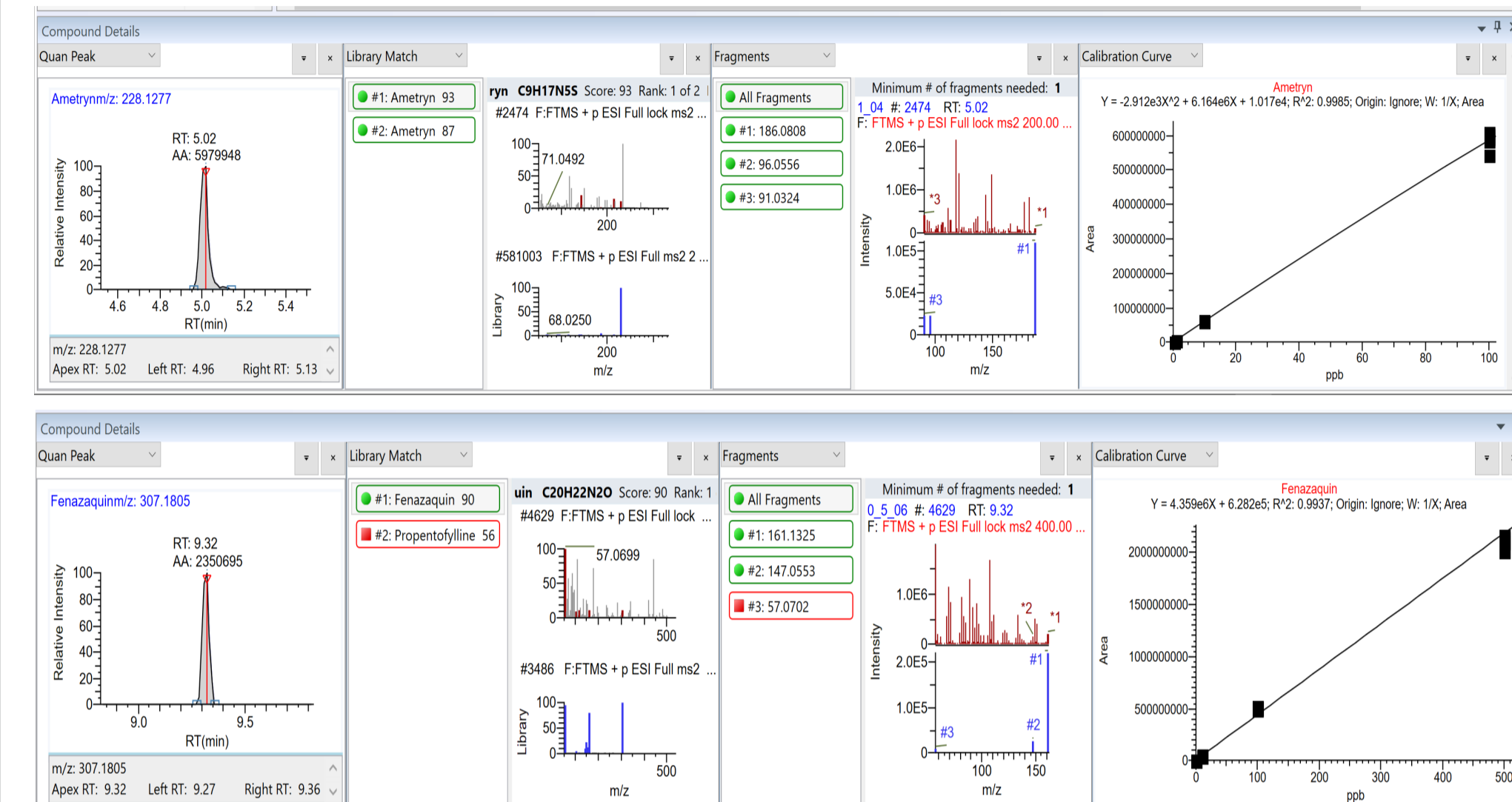
Figures 6: Quantitation ions and confirming ion in MMS in olive oil, along with calibration range from 0.5 to 100 (500) ppb in TraceFinder software for Ametryn @1ppb (top) and Fenazaquin 0.5ppb (bottom). The technique allows for confident quantitation and screening well below the MRL concentration.
