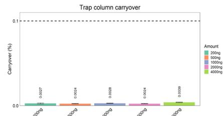
Figure 3. Trap column carryover after injection of HeLa protein digest with amounts from 200 to 4,000 ng, 3 replicates for each injection amount. The carryover was estimated based on the sum intensity of all quantified HeLa peptides.
