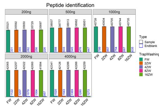
Figure 5. The number of peptides identified with the injection of 200 to 4,000 ng of HeLa protein digest and a blank injection afterward, 3 replicates. The trap column was washed with Fast Wash or ZebraWash (2, 4, 8, 16 cycles).
