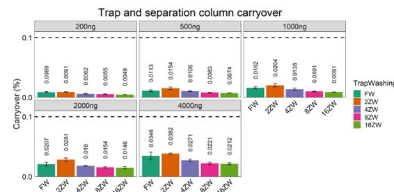
Figure 4. The level of overall carryover for different injection amounts and trap wash procedures, 3 replicates for each injection amount. The carryover was estimated based on the sum intensity of all quantified HeLa peptides.
