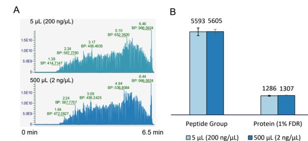
Figure 6. Total ion chromatograms (TICs) of 1 µg HeLa protein digest obtained after injection of 5 µL of 200 ng/µL sample and 500 µL of 2 ng/µL diluted sample onto the same trap cartridge (A) and the number of peptides and proteins identified from both injections using 180 samples per day (SPD) method (B).
