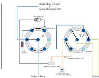
Figure 2. Schematic representation of the ZebraWash washing of the trap column with repeating plugs of strong and weak wash liquids
