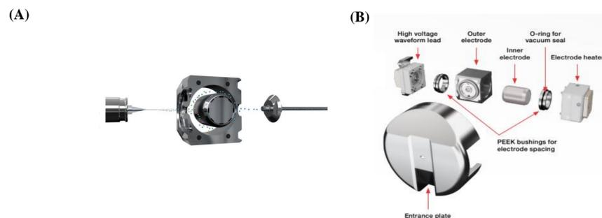
**Figure 5. FAIMS Pro interface enhances proteome coverage in single cell level by removing +1 charged ions; suppressing multiply charged peptides ions from single cell, allowing lower abundant peptides to be detected by MS.**
