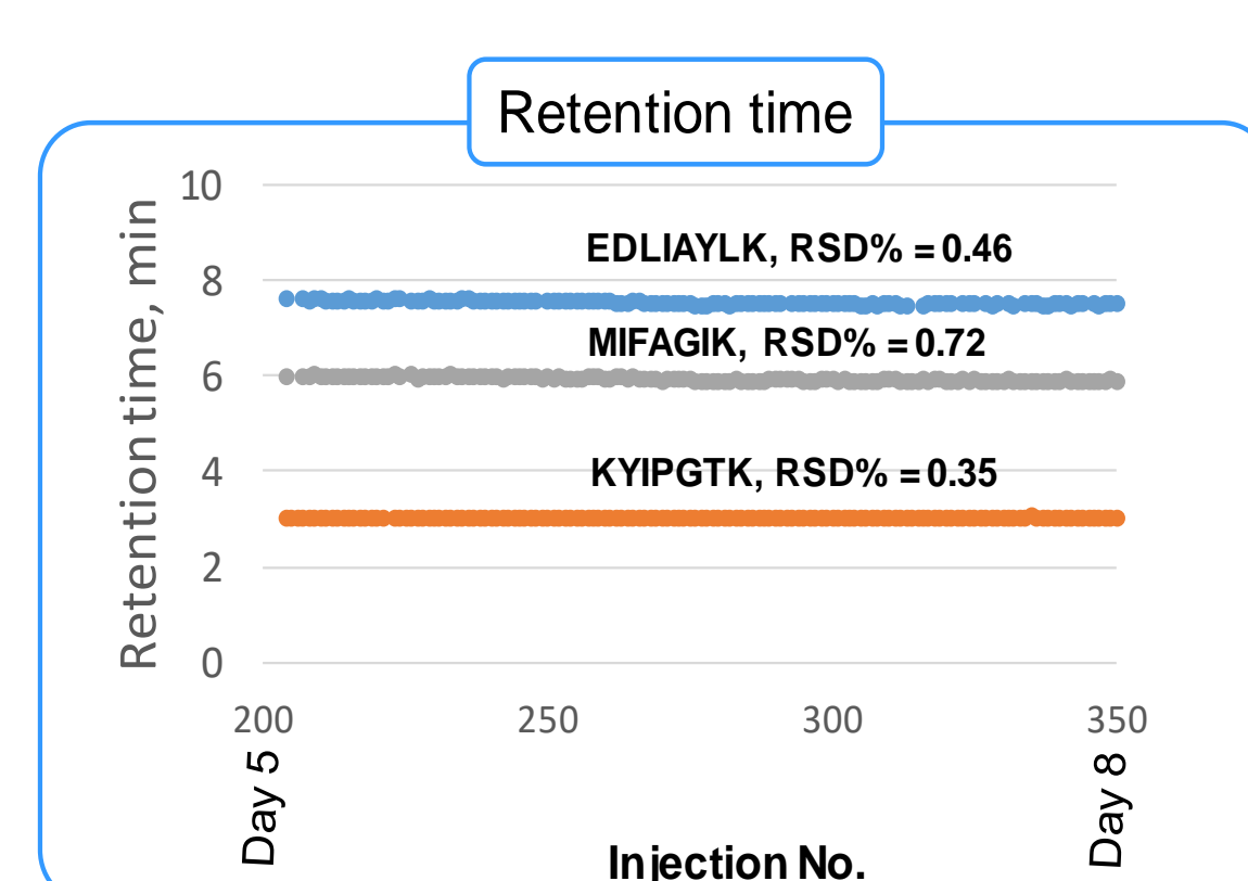
Figure 5. Retention time stability for capLC-MS analysis of CytC protein digest.
