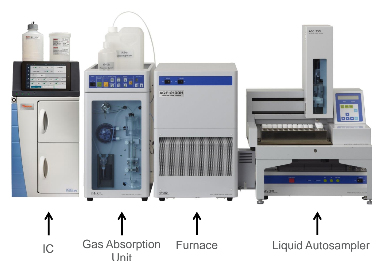
Figure 2. CIC system components.
