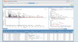
Figure 2: BioPharma Finder results showing the identification of a peptide based on the correlation between the observed MS/MS spectra and the theoretically predicted fragmentation pattern. High correlation and accuracy less than 3 ppm lead to a confident assignment. This peptide and many others can then be directly exported to Chromleon for monitoring as part of MAM.
