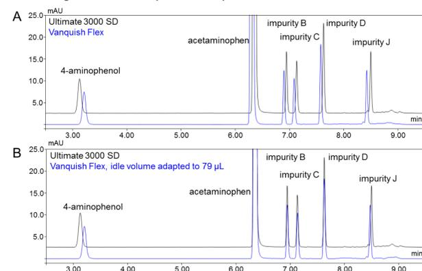
Figure 3. Acetaminophen assay before (A) and after (B) GDV adaption by sample loop and idle volume of the metering device in the Vanquish autosampler
