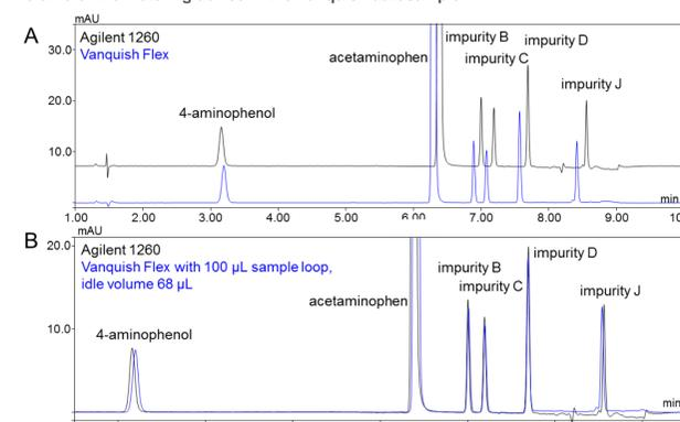
Figure 4. Acetaminophen assay before and after GDV adaption by static mixer exchange (A) and after applying a gradient prestart
