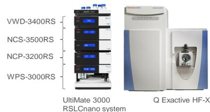
Figure 1. On-line 2D UltiMate 3000 RSLCnano system coupled with Q Exactive HF-X mass-spectrometer
