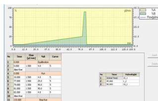
Figure 4. Gradient for the low pH reversed-phase peptide separation of 2 fractions in the 2nd dimension and corresponding TIC profiles
