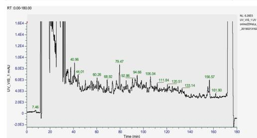
Figure 6. Gradient for low pH reversed-phase peptide separation of 4 fraction in the 2nd dimension on ES800A column
