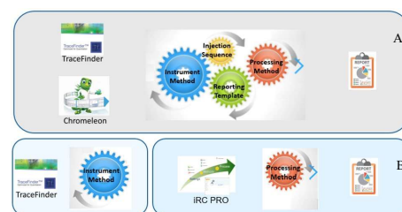
Figure 5. Workflow comparison between TraceFinder, Chromeleon and iRC PRO SW. A) Both TraceFinder and Chromeleon SW can use one software platform for data acquisition, processing, and reporting. When instrument method, processing method, reporting template and injection sequence are defined and ready, one click will initiate sample sequence submission with automated reporting. The strategy can provide a single, complete audit trail for acquisition, processing, and reporting, which would reduce and simplify audit preparation. B) iRC PRO SW has simple user interface. It can process raw data to reports, with behind-the-scenes built-in peak integration, calculation method, and reporting template. Setting up of the automated data processing can be started without learning the details of TraceFinder SW.
