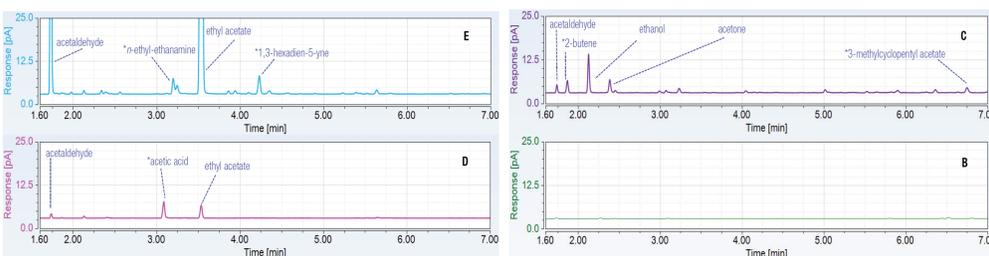
Figure 4. FID chromatograms: empty blank vial (B), salad wrap (C), sliced salami wrap: lid (D) and tray (E).
