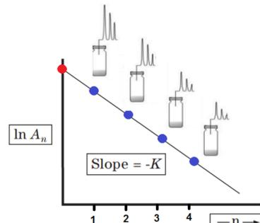
Figure 2. Principle of the MHE extraction.
