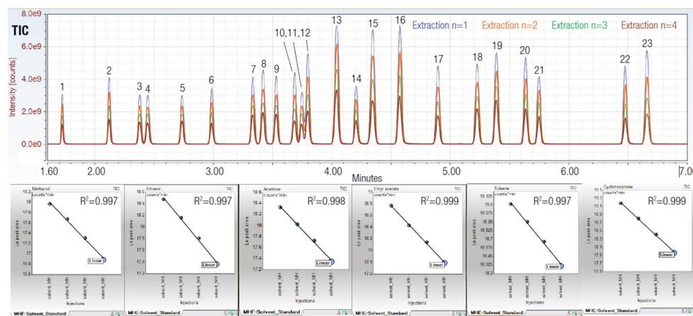
Figure 3. Full scan TIC chromatogram of reference standard and corresponding MHE calibration curves for selected compounds.
