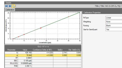
**Figure 6:** Calibration plot obtained for fluorine measured as Ba.F
