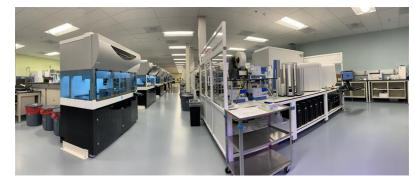
Module 1—Array samples Input: 378 tubes Output: Four 96 well DWP
