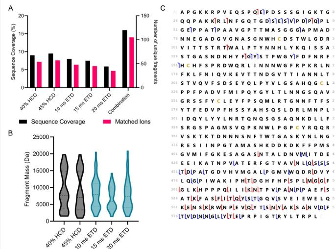
**Figure 5.** AAV6 VP2 subunit characterization. A single LC run was used for MS<sup>2</sup> fragmentation. Combined refers to the cumulative values of 45% HCD and 10 ms ETD. A) Sequence coverage and number of matched fragment. B) mass distribution for matched fragments. C) Combined HCD and ETD fragmentation map (16% sequence coverage).
