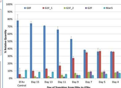
The timing of transition from EFA+ to GTA+ makes it possible to target specific glycosylation profiles. Modulating G0F from 78% down to 36%, while increasing G1F (1 and 2) and increasing G2F.
