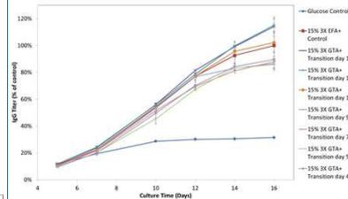
DG44 titer comparison between feeding conditions. Titrers were similar with both EFA+ and with the use of or when transitioning to GTA+, 100% titer is the titer of 15% 3X EFA+ on day 16. Titer results indicate that the use of and transition to GTA+ does not negatively affect protein production.
