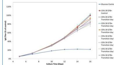
Titer comparison between feeding conditions. Titrers were similar with both EFB+ and with the use of or when transitioning to GTB+, 100% titer is the titer of 15% 3X EFB+ on day 16. Titer results indicate that the use of and transition to GTB+ does not negatively affect protein production.
