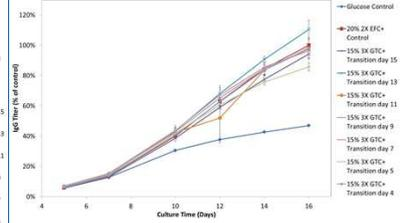
Titer comparison between feeding conditions. 100% titer is the titer of 15% 3X EFC+ on day 16. Titer results indicate that the use of and transition to GTC+ does not negatively affect protein production.
