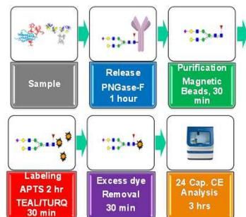
Glycan analysis workflow – 3 hours of hands on time, 7-9 hours to process and analyze 96 samples with no vacuum centrifugation.
