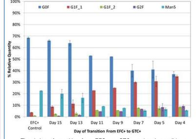
The timing of transition from EFC+ to GTC+ makes it possible to target specific glycosylation profiles. Modulating G0F from 68% down to 37%, while increasing G1F (1 and 2) and increasing G2F.
