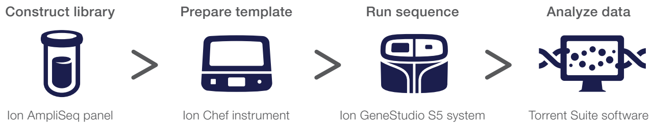
Figure 1. Targeted NGS workflow using the Ion GeneStudio S5 Series System. Ion AmpliSeq™ libraries are prepared manually or with the Ion Chef™ System. Libraries are then placed in the Ion Chef System for emulsion PCR, enrichment, and loading onto Ion S5™ Chips.
