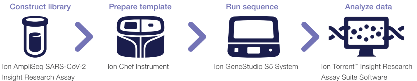
Figure 1. Workflow for targeted NGS on the Ion GeneStudio S5 System. Ion AmpliSeq™ libraries can be prepared manually or with the Ion Chef™ Instrument for emulsion PCR, enrichment, and loading onto Applied Biosystems™ Ion S5™ chips.
