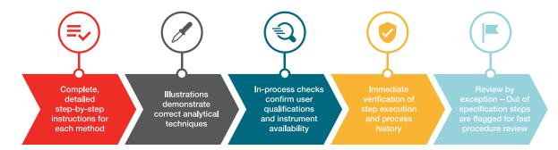
The Laboratory Execution System (LES) software guides analysts through each step of a method to ensure compliance to the SOP and captures the complete process history.
