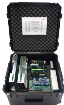
Figure 2 The strategic electronics spares kit. Dimensions: 65 × 65 × 36 cm.
