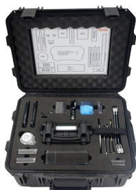
Figure 1 The standard spares kit with the tested ion source supplied in its own internal carry case. Dimensions: 55 × 42 × 26 cm.
