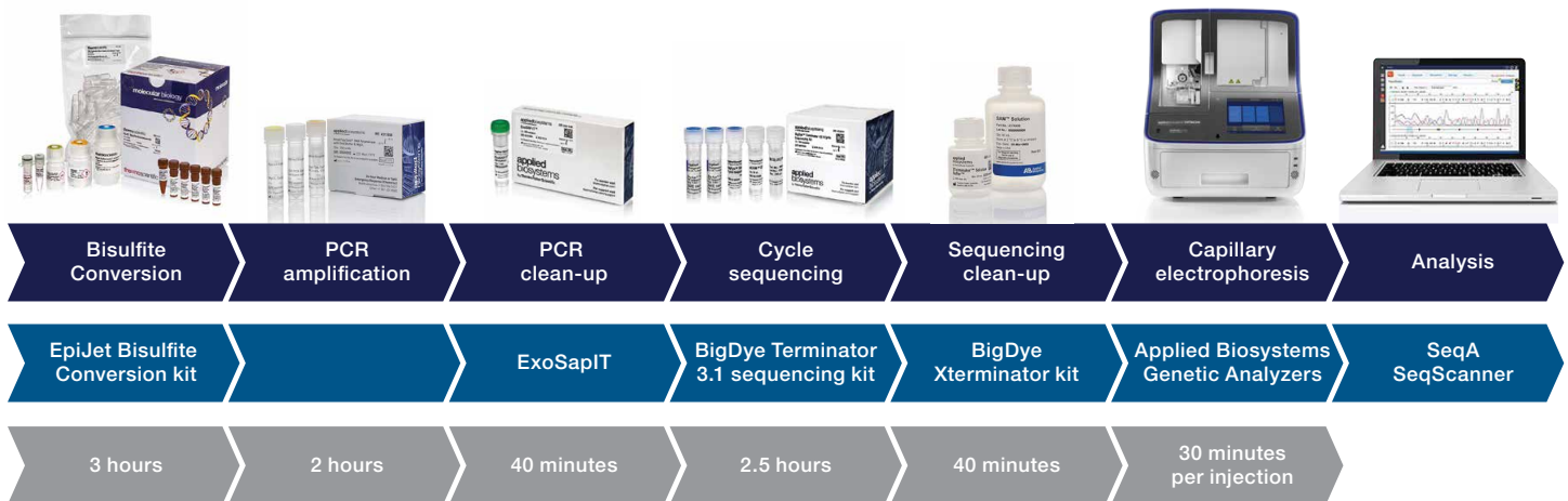
Figure 2. Workflow for methyl DNA analysis using Sanger sequencing.
