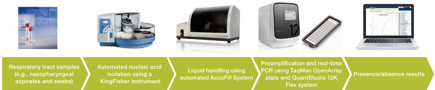
Figure 1. Workflow for detection of respiratory tract pathogens. The workflow shows extraction of total nucleic acid from respiratory tract samples using a KingFisher instrument and the Applied Biosystems™ MagMAX™ Viral/Pathogen Ultra Nucleic Acid Isolation Kit, followed by preamplification and then real-time PCR analysis using the TaqMan OpenArray plate on the QuantStudio 12K Flex system. Results provide a detected/not detected call for each of 42 targets that include bacteria, RNA and DNA viruses, and fungi, as well as for optional B. atrophaeus extraction and Xeno RNA spike-in controls.
