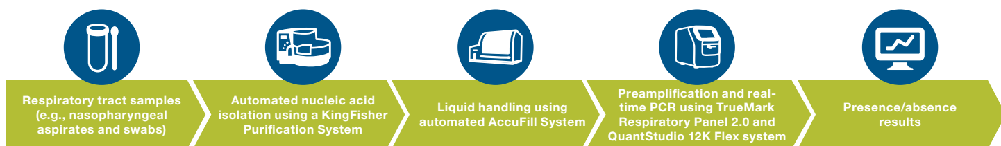
Figure 1. Workflow for detection of respiratory pathogens. The workflow shows extraction of total nucleic acid from respiratory tract samples using a KingFisher Purification System and the Applied Biosystems™ MagMAX™ Viral/Pathogen Ultra Nucleic Acid Isolation Kit, followed by pre-amplification and then real-time PCR analysis using the TrueMark Respiratory Panel 2.0, OpenArray Plate, on the QuantStudio 12K Flex system. Results are provided in the form of a presence or absence call for each of the respiratory pathogen targets that include bacteria and RNA and DNA viruses.
