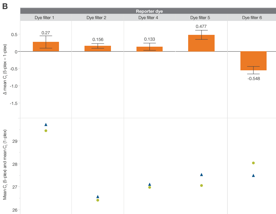
Figure 4. TaqPath DuraPlex 1-Step RT-qPCR Master Mix has characteristics that are ideal for multiplexing reactions. (A) TaqPath DuraPlex master mix can effectively amplify from targets of varying input in a multiplex reaction. The reaction was run on an Applied Biosystems™ QuantStudio™ 5 Real-Time PCR System with an Applied Biosystems™ probe. (B) TaqPath DuraPlex master mix maintains performance when scaled up from a single-target reaction to a multitarget reaction. Dyes and associated filters: filter 1 = FAM dye; filter 2 = VIC dye; filter 4 = JUN dye; filter 5 = cyanine 5; and filter 6 = cyanine 5.5.
