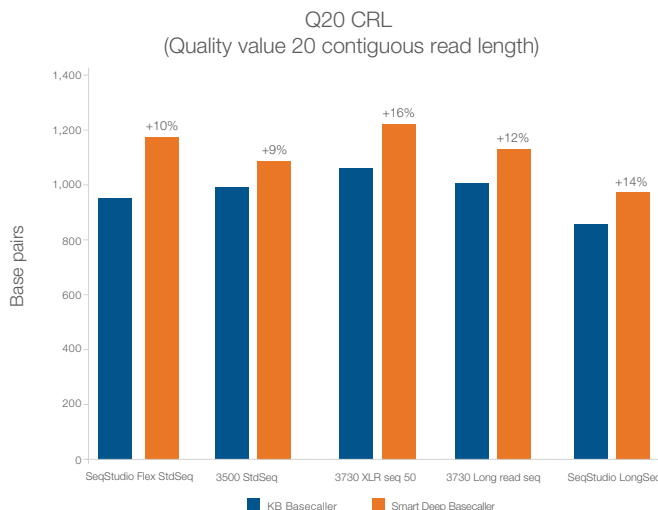
Figure 1. Increased throughput with longer reads. By producing more accurate basecalls with higher quality scores, Smart Deep Basecaller generates longer read lengths after quality trimming. Datasets were provided for the Applied Biosystems™ SeqStudio™ Flex Genetic Analyzer, Applied Biosystems™ 3730 DNA Analyzer, Applied Biosystems™ SeqStudio™ Genetic Analyzer, and Applied Biosystems™ 3500 Genetic Analyzer. The data show read lengths were increased 9–16%. The advanced algorithm in Smart Deep Basecaller allows for greater accuracy in the 5'- and 3'-ends to optimize the number of bases per read.
