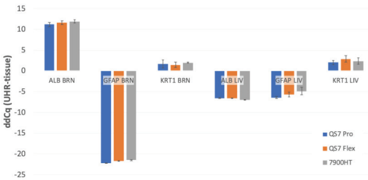
Figure 2. Comparison of ddC_q data between QuantStudio 7 Pro, QuantStudio 7 Flex, and 7900HT Real-Time PCR Systems. Data show equivalent relative expression level of ALB , GFAP , and KRT1 in the cDNA of total brain RNA and total liver RNA (data generated in Microsoft ® Excel ™ software).
