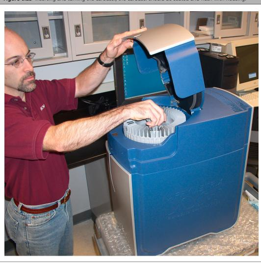
Figure 6.23 Inserting and turning the carousel; the carousel should be seated and flush with housing.
