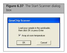
If you want to skip the warm-up period before scanning the first probe array, keep the default check in the Arrays at room temperature box.
