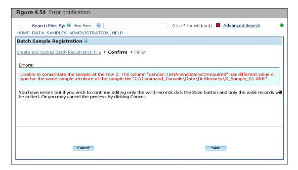
The error messages indicate problems such as bad barcodes, problems with registering multiple arrays on a sample, etc.
