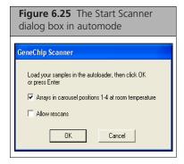
If you want to skip the warm-up period before scanning the first probe array, keep the default check in the First 4 arrays at room temperature box.
