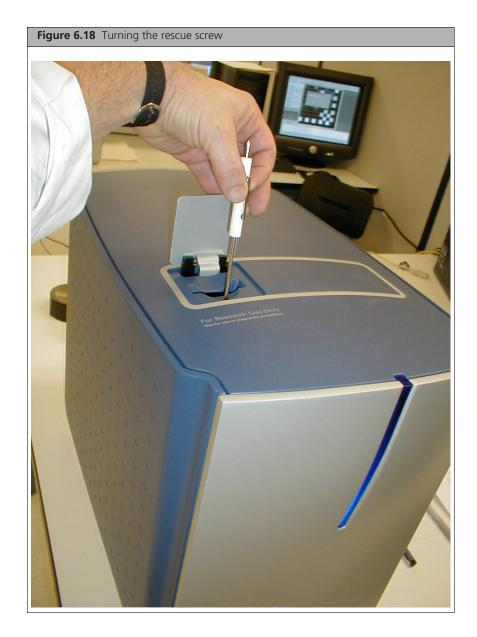
Note that the screw is fine pitched and requires a number of turns. Stop if you encounter screw resistance. Do not over torque.
