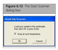
If you want to skip the warm-up period before scanning the first probe array, keep the default check in the Arrays at room temperature box.
