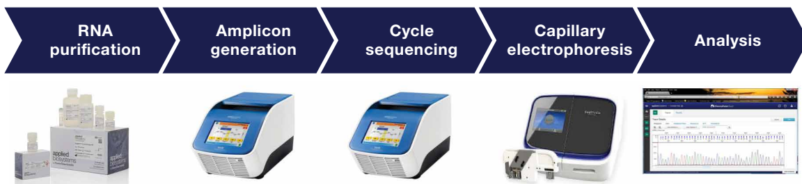
Figure 1. Workflow for detection of SARS-CoV-2 lineages using Sanger sequencing. RNA is purified from samples using standard techniques. cDNA is synthesized from the RNA, and specific M13 sequence–tagged amplicons are generated by PCR. The amplicons are sequenced in the forward and reverse directions using universal M13 primers and the BigDye Direct Cycle Sequencing Kit. The sequencing reactions are cleaned using the BigDye XTerminator kit and subjected to CE. The resulting sequencing traces can be analyzed and compared to reference SARS-CoV-2 sequences to determine if the lineages are present.
