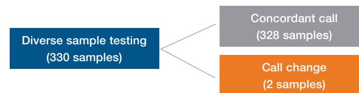
Figure 3. RT-qPCR results comparing new and on-market products for a large diverse sample set. Of the 330 calls, two calls were changed: one from positive to negative ( C_t of 35.3 using on-market products to a C_t of 40 using newly developed products) and one from negative to positive ( C_t of 38.6 using on-market products to a C_t of 23.9 using newly developed products).
