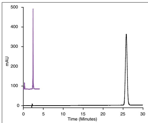
Figure 2: Chromatograms of 100 µg/mL of zidovudine separated on a Synchronis C18 1.7 µm, 50 x 2.1 mm column (top chromatogram), and on a Synchronis C18 5 µm, 250 x 4.0 mm column (bottom chromatogram)
