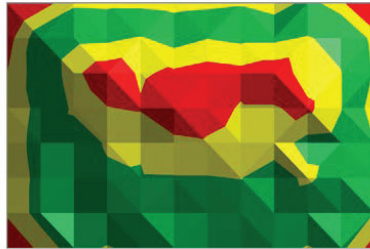
Figure 3. Cell viability. Variance in cell viability is minimized in plates with a built-in perimeter moat, compared to those with no moat. The Nunc Edge 2.0 plate with the larger built-in moat more effectively improves cell viability and consistency across the entire plate.
