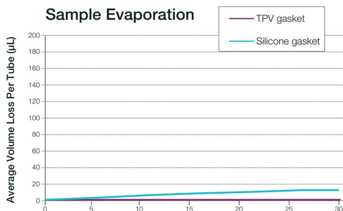
Figure 1. Average sample evaporation at room temperature in tubes with either TPV or silicone gaskets/closures.
