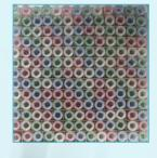
Since many samples are only 1.0mL or less, this storage system uses 1.0mL tubes in a 13 x 13 (169 tubes) array, to double existing freezer space capacity
