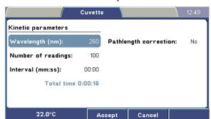
**Kinetic** Use the **Kinetic** session to perform a kinetic measurement on a cuvette.
