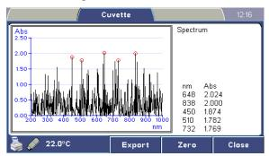
DNA/RNA sessions: the measured spectrum is displayed along with measured and calculated results.
