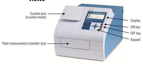
Figure 2–2. Multiskan GO with cuvette front view
