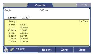
The measurement time is displayed to the right of each result. Up to 24 measurement results are simultaneously displayed on the screen. However, the instrument stores up to 100 latest measurements, which you can retrieve by exporting the single measurement to the USB memory device or by printing the results.
