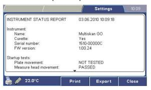
The status report provides current information on the instrument status, including the instrument model and serial number, firmware version, current temperature and other parameters.
