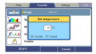
The temperature setting range is 10–45°C with a resolution of 1°C. When the heating is on and the temperature set, the target temperature is displayed on the info text bar (see below).
