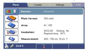
The **Plate** menu contains settings for the session name, plate format, measurement area, plate incubation and shaking, and the measurement type.
