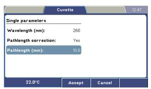
The **Single** submenu contains the following parameters:
