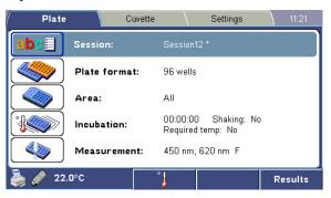
The asterisk (\*) by the session name indicates unsaved results. These are retained until new results are generated. To store results for later use, you should save them in the instrument's memory, export them to a connected USB memory device or print them on a connected USB printer.
