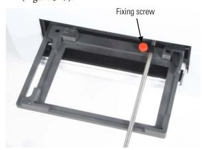
Figure 3–9. Plate carrier pulled fully out
