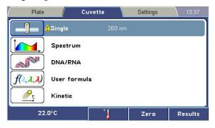
Cuvette sessions or measurement results cannot be stored in the instrument's memory. You should export or print measurement results if you wish to use them later. The instrument memorizes the most recent measurement parameters and results for each predefined session type.
