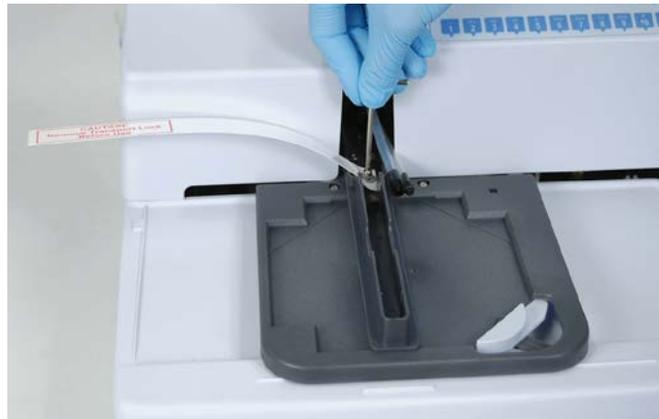
**Figure 42.** Fastening the transport lock
