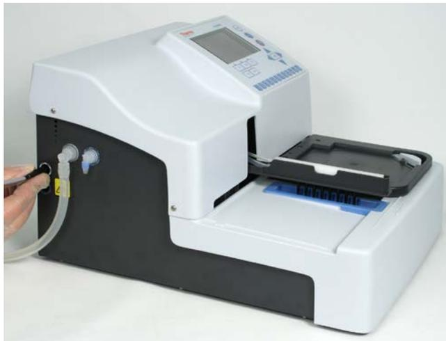
**Figure 16.** Connecting the liquid sensor cable
