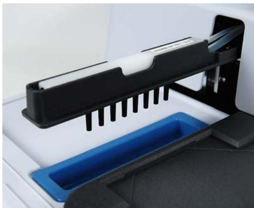
**Figure 11.** 1x8 wash head properly inserted
