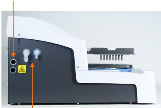
Connectors for liquid container tubes,
