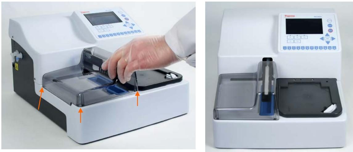
**Figure 20.** Installing the aerosol cover
