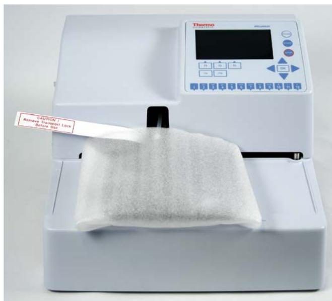
**Figure 43.** Transport lock and tag fitted
