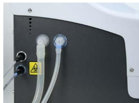
**Figure 17.** Liquid bottle tubings connected to the instrument
