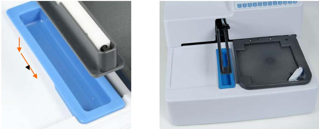
Figure 7. Priming vessel installation
