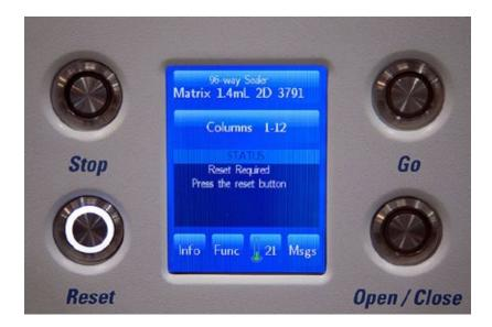
Press the **RESET** pushbutton. The instrument will initialize and, if foil is loaded and the compressed air supply is connected, the sealer will start to warm up.
