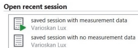
Figure 44. A session with measurement data (green icon) and without measurement data (no icon).
