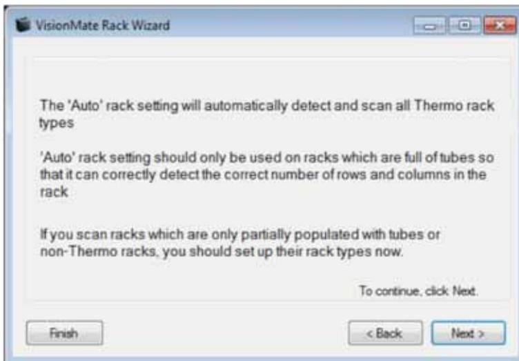
At this point place a **fully populated** rack of tubes onto the scanner.
