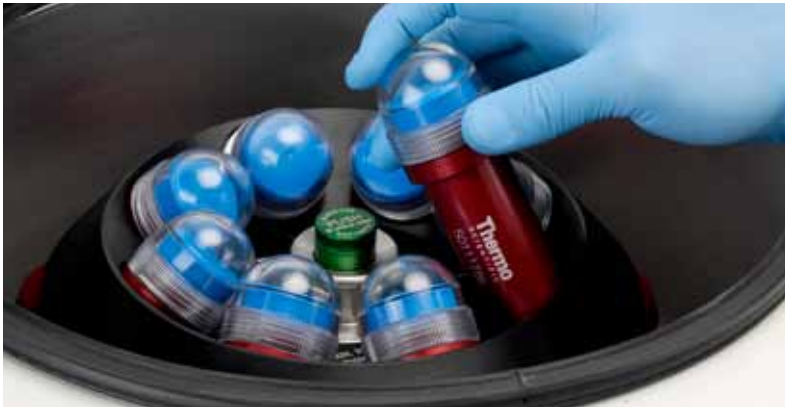
Figure 2: Preferred centrifuge configuration with 8x50 mL individually sealed fixed angle rotor in non-refrigerated Thermo Scientific 1-Liter general purpose centrifuge
