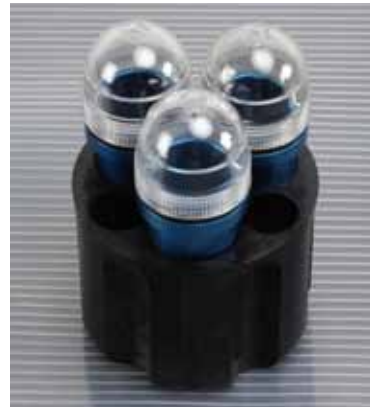
Figure 3: Alternative centrifuge configuration with individually sealed adapters for TX-750 swinging bucket rotor in Thermo Scientific 3-Liter refrigerated general purpose centrifuge
