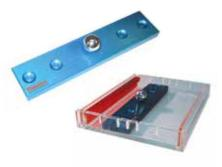
Three-point leveling platform ensures flat casting and running surface
