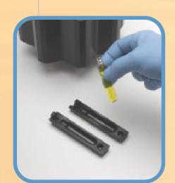
Fill tube to specified volume and balance to specified tolerance.
