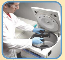
Follow manufacturer's instruction for locking mechanism, securing the rotor.
