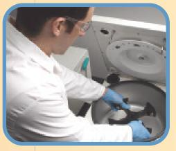
Confirm rotor is locked down before pressing start.
