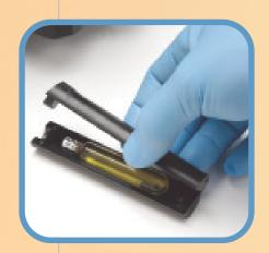
Place tube into cartridge or rotor cavity, ensuring tube fits perfectly into the cavity.
