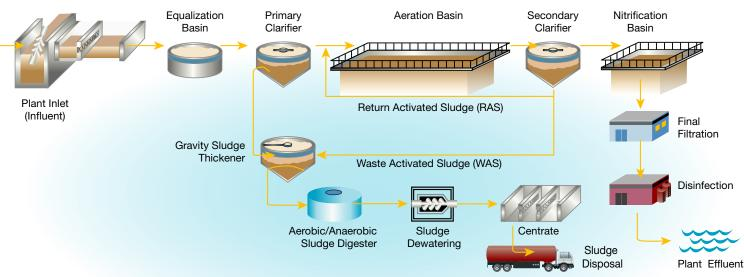
Figure 1: Wastewater treatment process demonstrates the five basic processes described above.
