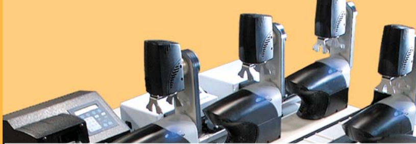
Unique distributed motion robotic technologies give the Dimension4 automation platform its exceptional throughput and flexibility. (Clockwise, l to r) Thermo Scientific Vertical Array Loader, Thermo Scientific Flip Movers, Thermo Scientific Linear Plate Transport.
