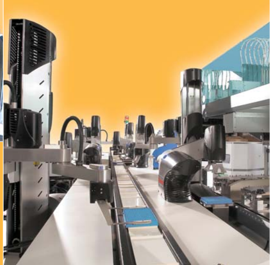
Unique distributed motion robotic technologies give the Dimension4 automation platform its exceptional throughput and flexibility. (Clockwise, l to r) Thermo Scientific Vertical Array Loader, Thermo Scientific Flip Movers, Thermo Scientific Linear Plate Transport.
