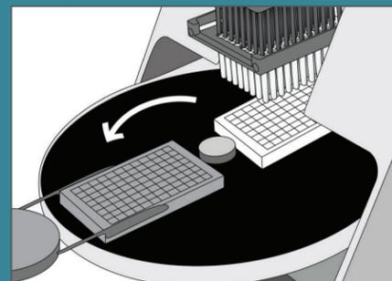
3 New plate is automatically moved into loading position for further processing, which ensures seamless purification without any delay between steps and use any number of plates.
