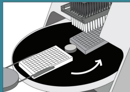
1 Plate is loaded into loading position.
