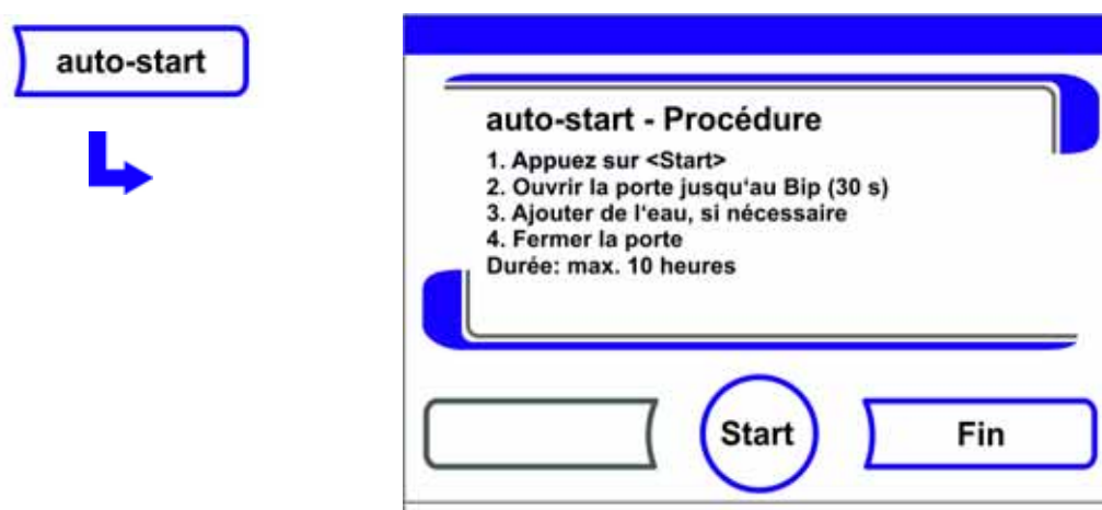
Figure 5-20 Activer la routine auto-start
