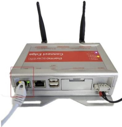
**Note:** If using Wi-Fi, attach the gateway Wi-Fi antennas. If using cellular, attach the cellular antennas.
