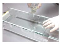
3. Capillary action wicks polyacrylamide between the glass plates for a perfect bubble free gel.
