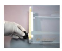
2. Pour the acrylamide solution onto the bottom plate while slowly sliding the top plate into position.
