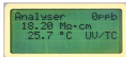
Picture shows Analyser mode when IC system cable is connected on the Dionex IC Pure system.
