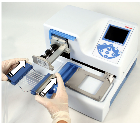
Figure 4–11. Inserting the dispensing cassette
