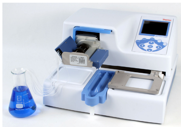
Figure 4-19. Rest position of the dispensing cassette
