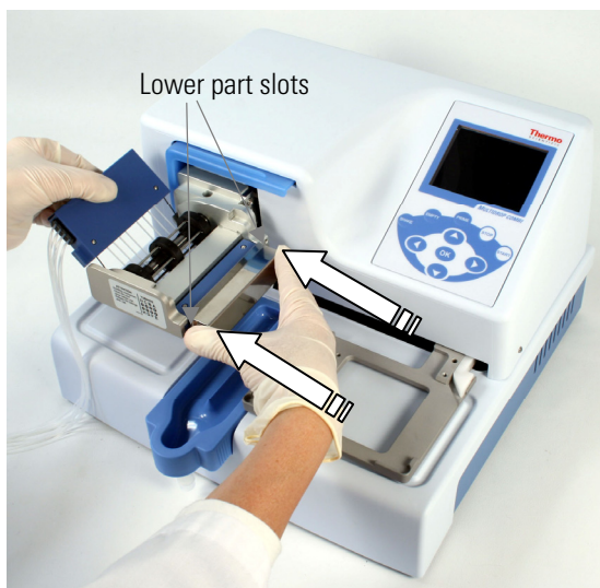
Figure 4–12. Inserting the lower part of the dispensing cassette into its slots
