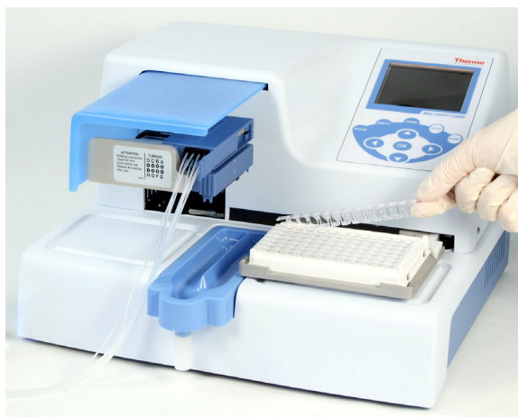
Figure 6–49. Removing the filled microstrip to be weighed
