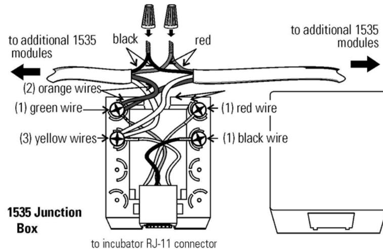
**Figure 6-2.** RS485 Wiring
