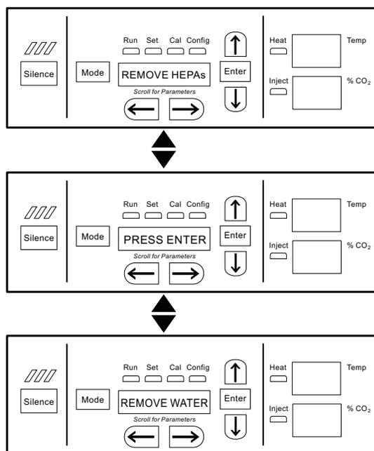
**Figure 5-14.** Displays with IR Sensor Removed
