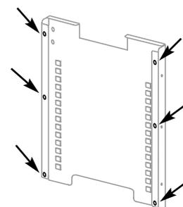
**Figure 1-10.** Grommets on back of duct sheet
