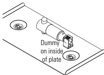
**Figure 5-12.** Dummy Sensor
