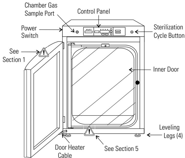
**Figure 1-1.** Steri-Cycle Components
