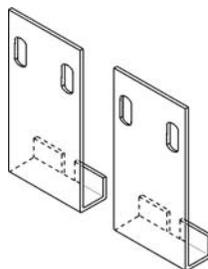
Two stacking brackets (shown at left) are included in the parts bag shipped with each incubator.
